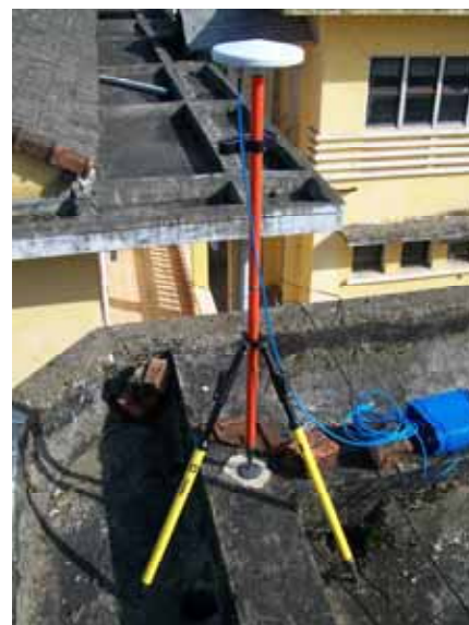
Figura 1 - Trimble GPS antenna on site on the IMOLA CGT benchmark established on the roof of the project office, to link IMOLA CGT and TeMa networks.
