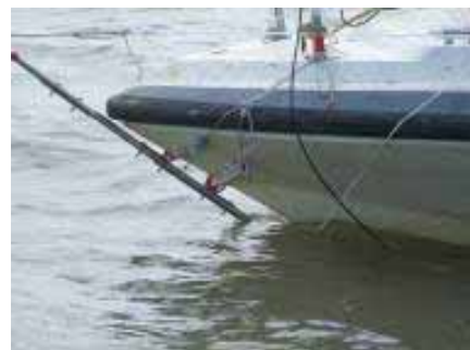
Figure 3 - Design of the ADCP installation on the hydrographic vessel used for survey
