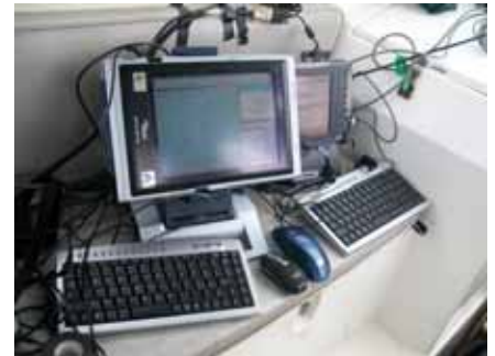
Figura 4 – Computerized control console of the RESON PDS2000 hydrographic suite for bathymetric survey
